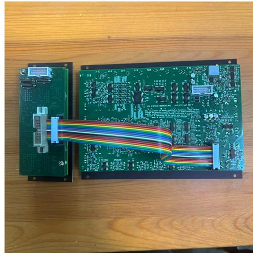
*Connecting an expander—use whichever end is most convenient*
