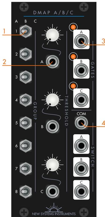
1. Group Selection – These switches place stages 1–8 of the connected Discrete Map in groups A (left), B (center), or C (right).
